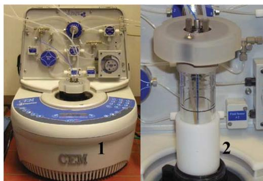
Figure 1. Voyager platform (1) and 80 mL glass vessel (2).
