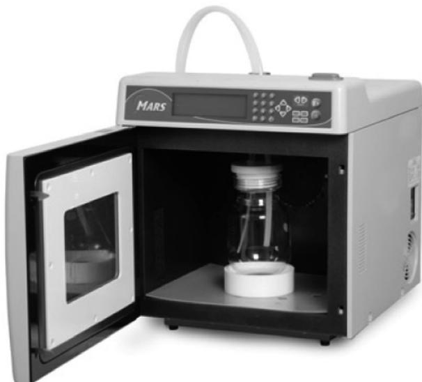
**Figure 2.** Flow-through reactor (2 L) inside the microwave cavity.
