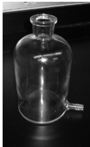
**Figure 1.** Prototype of the 2 L reaction vessel.
