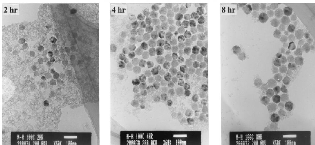
Figure 3. Morphology of  $\gamma\text{Fe}_2\text{O}_3$  via MW irradiation for 2 h (left), 4 h (middle), and 8 h (right).<sup>5</sup>
