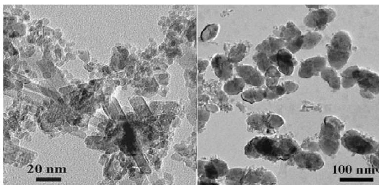
**Figure 2.** MION prepared via oil bath (left) and MW irradiation (right).<sup>2</sup>
