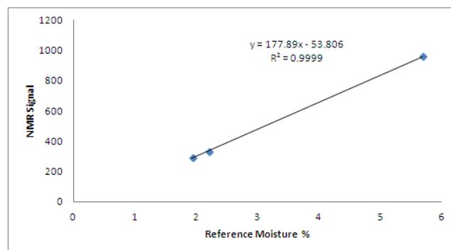
Figure 2: Moisture calibration curve
