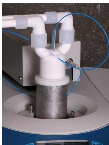
Figure 3. Sub-ambient Reaction Accessory.
