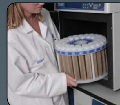
2. Place the vessel in the turntable and place in the system.
